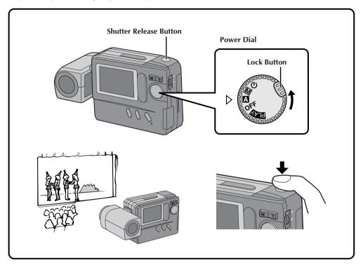
Turn the Power Dial, while pressing its Lock Button, to "A".
